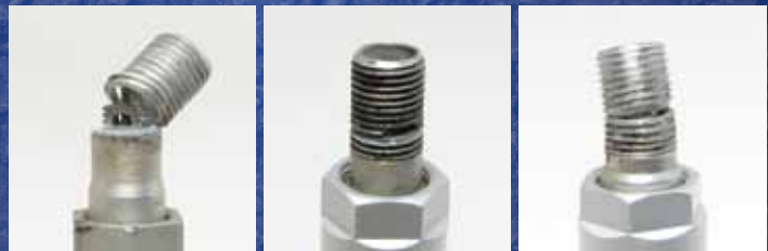
Galvanic corrosion causes TPMS failures.
