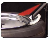
Patented laser imaging technology scans wheel profile for precise tool placement.
