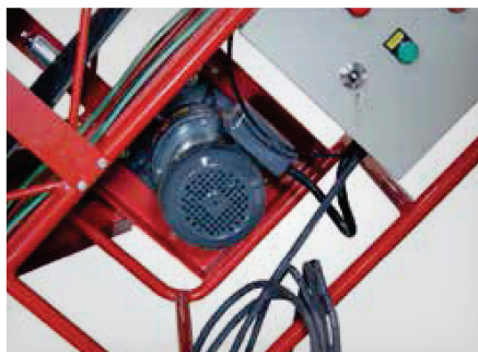
Tire conveyor motor 1 HP or 1,5 HP (depending on the conveyor model)
