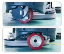
The SafetyGlide<sup>™</sup> Deck automatically moves in line with the path of the rear squeegee when the steering wheel turns.
