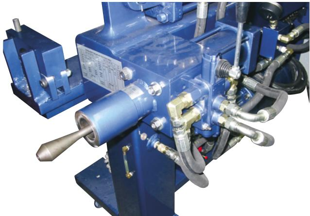
Provides rapid set-up time and high degree of accuracy for both I.D. and O.D. expansions including slip fits, flare, inner flaring with segment type tooling. This unit can expand muffler nipples and works closer to bend than the expander. You merely snap on the proper tooling segment set, dial in the desired dimensions on the micrometer-type barrel, which is calibrated in 1/64" insert and jog the hydraulic control handle to complete the expansions.
