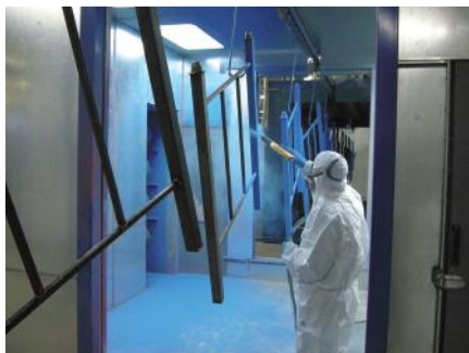
Baked powder coating paint facility.
