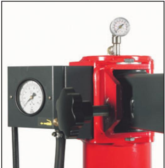
**GB** The rounded column is also a reservoir tank for the extra air needed when is used the tubeless inflation system (TI).
