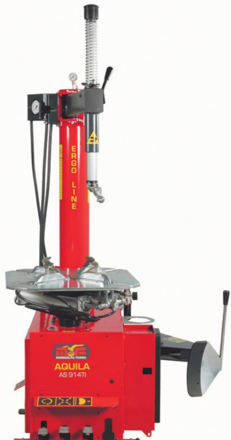
**GB** The help device (accessory) can be used to assist the operator in mounting and demounting difficult tyres as the low profile tires, Run Flat Tires and Pax tyres.
